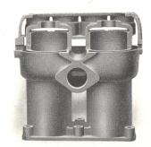
mensions are provided for both combustion chambers and valve pockets.
